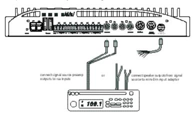
High-level MiniDin input connections
